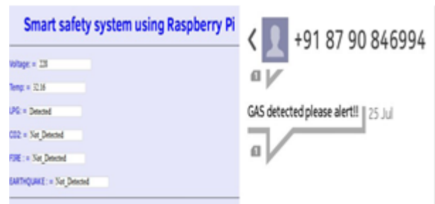
Fig. 8 Monitoring of LPG gas sensor.
