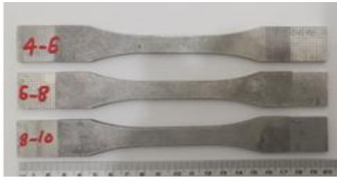
Figure 1: Image of test specimens after shot peened
