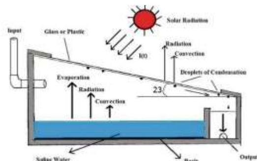
**Fig.3. Working on the conventional single slope solar still**
