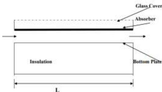
**Figure1: Conventional Solar Air Heater**
