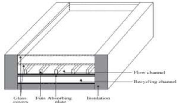
**Figure 2: Schematic diagram of double pass internally finned solar air heater**
