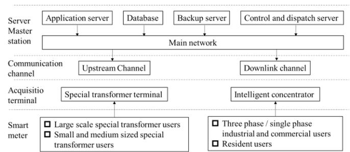
**Figure 1.** Structure diagram of power consumption information acquisition system.
