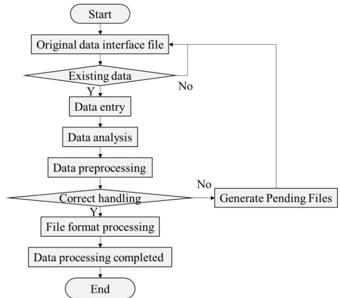
Figure 5. Data analysis process flow.
