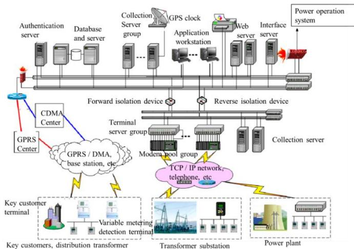
Figure 4. Master station network topology.
