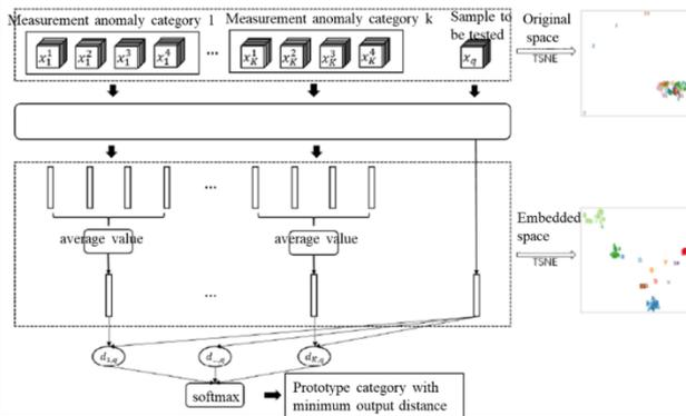
**Figure 7.** Measurement anomaly diagnosis model based on small sample learning.
