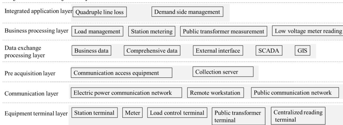
**Figure 3.** Overall structure of the system.
