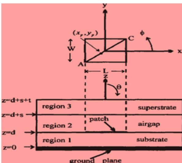
Figure:2- Geometry of the rectangular shape antenna used by the
