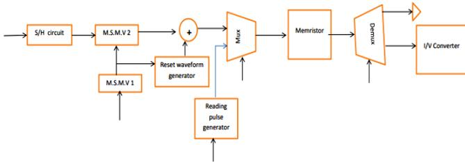
**Figure 2. Basic Memory cell with S/H- Sample and Hold Circuit, MSMV-Multi State Multi Vibrator, I-Current, V-Voltage.**
