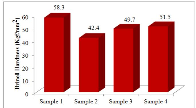
Figure 3: Brinell hardness of as cast Al-Cr alloy samples
