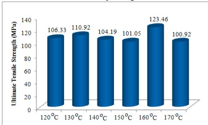
Figure 2: Ultimate Tensile Strength of artificially aged 99.5Al-0.5Cr alloy
