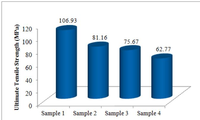
Figure 1: Ultimate Tensile Strength of as cast Al-Cr alloy samples
