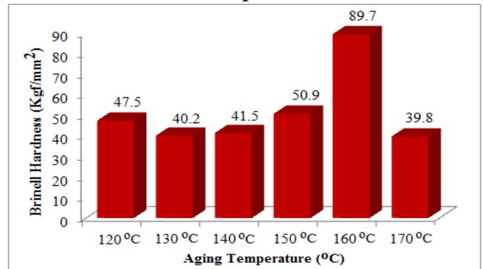
Figure 4: Brinell hardness of artificially aged 99.5Al-0.5Cr alloy
