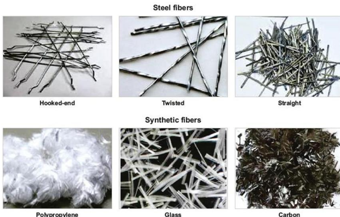
Figure 4. Synthetic and steel fibers used in concrete formulations
