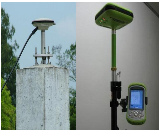
Figure.No 4.a) Base station set up b) RTK-GPS Rover set up
