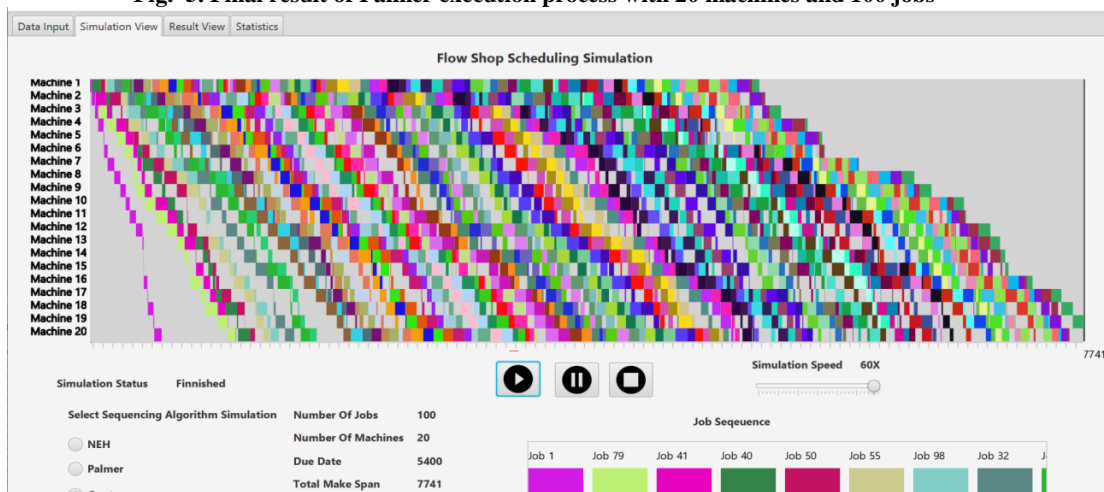
Fig. 6. Report result of NEH, Palmer, and Gupta execution process with 20 machines and 100 jobs
