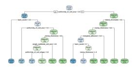
For breast cancer diagnosis a predictive model is developed using a decision tree. In this paper a decision tree is used for classification to establish the model. [9] To prepare training and test data 10-fold cross validation is used. After data preprocessing (CSV format) using R studio, the algorithm is employed on the dataset, subsequently the data are classified into "benign" or "malignant" based on the endmost outcome of the decision tree that is constructed.
