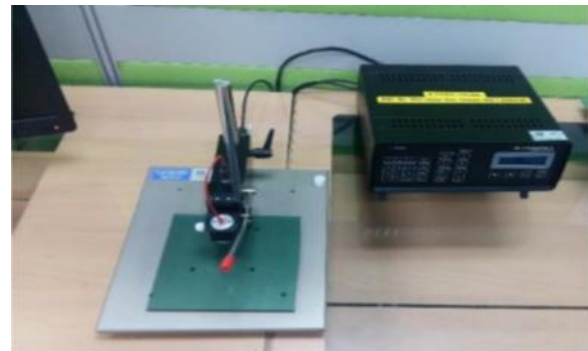
Figure 4: JANDEL In-Line 4 Point Probe test equipment
