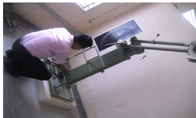
Figure 2 Measurement of impact strength by Charpy Testing Machine
