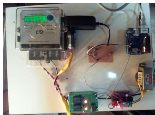
Figure 10: It showing the electricity theft prediction with instant billing using android application
