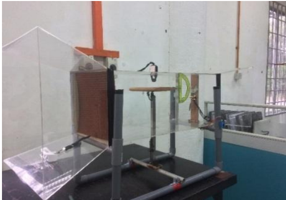
Figure 1: The construction of a smallscale wind tunnel
