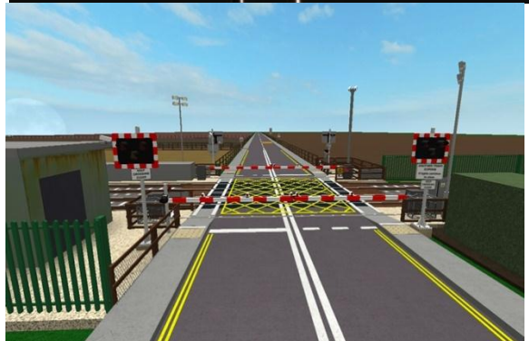
Figure 7: Level Crossing when gates are closed
