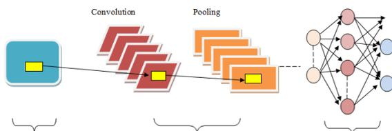
Figure 2: Architecture of Deep CNN
