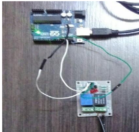
Figure 3: Connection between the Relay switch and Arduino
