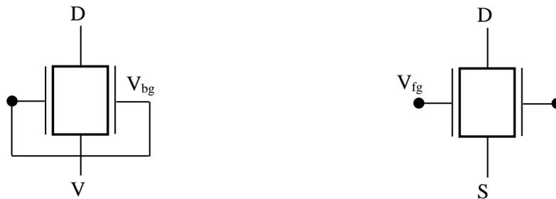
(a) Shorted Gate FinFET ( $V_{fg} \neq V_{bg}$ ) (b) Independent Gate ( $V_{fg} \neq V_{bg}$ )
