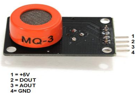
Figure. No. 01. Alcohol sensor MQ-3
