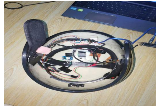
Fig. 5. A complete circuit mounted inside a helmet
