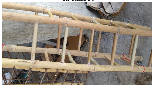
Fig. 3.8 This picture indicate the interlocking system used for connecting bamboo.
