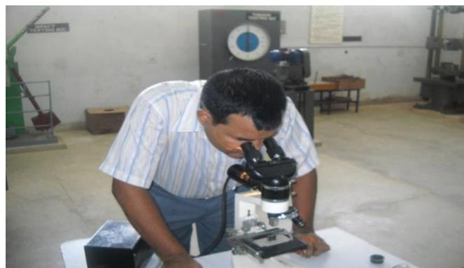
Figure 1 Measurement of Weld Bead Dimensions with Metallurgical Microscope
