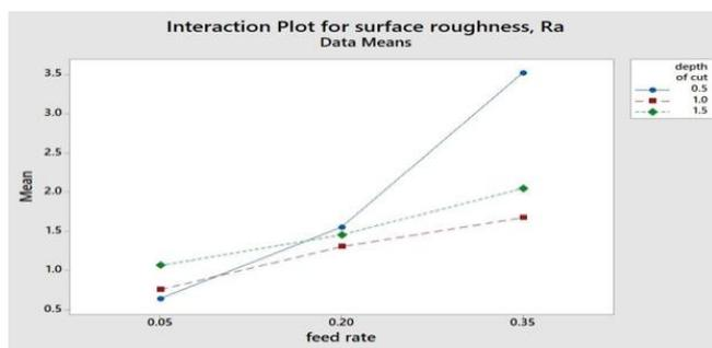
Fig. 7. Interaction graph for  $Ra$  between  $f$  and  $d$ .
