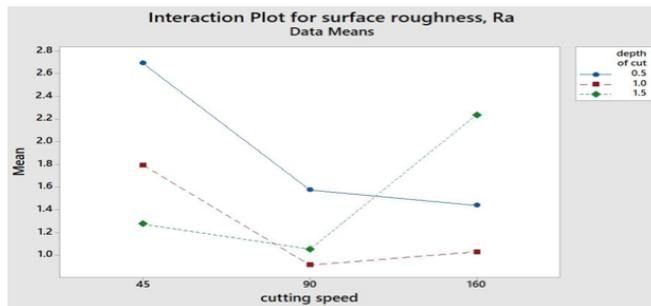
Fig. 6. Interaction graph for Vs between  $Ra$  and  $d$ .
