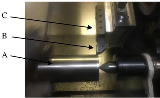
Fig. 2(a). The work piece (A), cutting tool (B) and dynamometer Setup (C)
