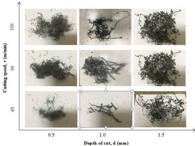
Fig. 9. The chips formed after turning process cutting speed against depth of cut.
