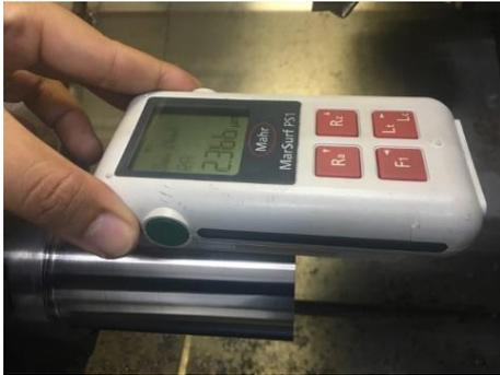
Fig. 2(b). Surface roughness measurement
