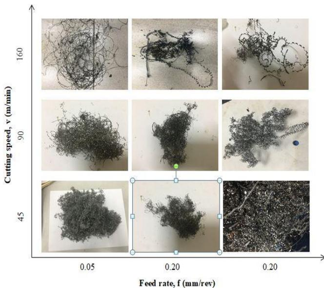
Fig. 10. The chips formed after turning process cutting speed against feed rate
