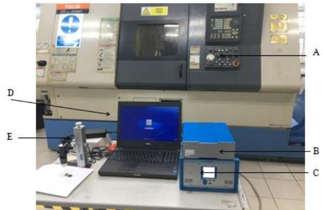
Fig. 1. The experimental setup for (A) CNC Turning Machine (B) Data Acquisition System (C) Multichannel Charge Amplifier (D) Laptop (E) Dino-Lite camera.
