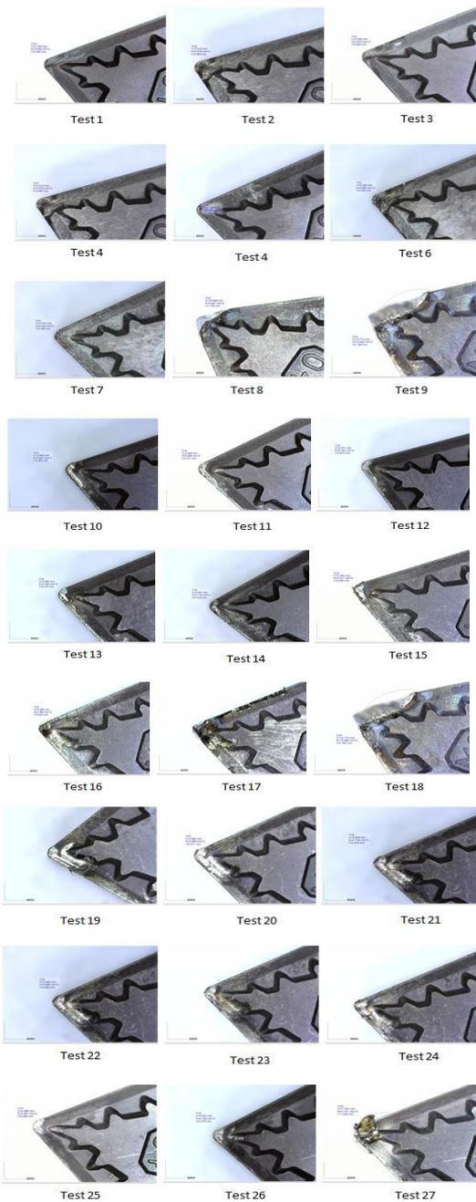
Fig. 8. The tool wear with measured nose radius after turning process for experimental tests 1 to 27.
