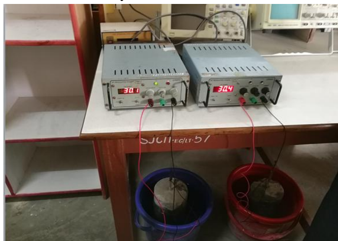
Fig.11 Accelerated corrosion test
