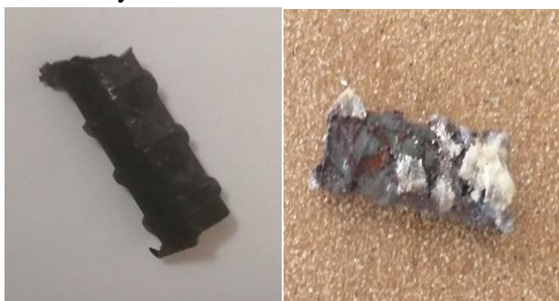
Fig.2 Mild steel before and after corrosion
