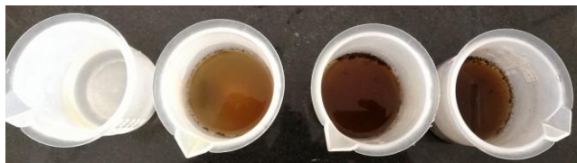
Fig.1 Containers with 1N NaCl each and 0g, 0.25g, 0.5g, 0.75g concentration of extract from left to right
