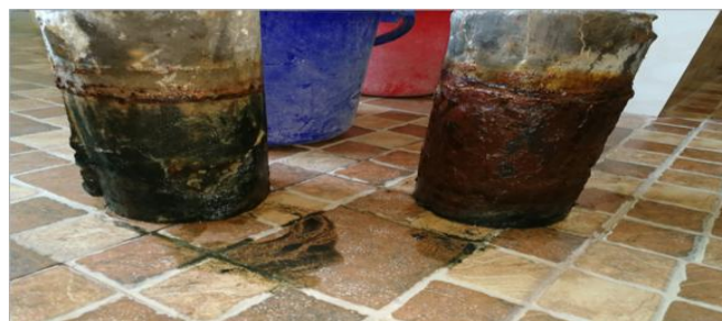
Fig.12 Reinforced concrete specimens after 10 days of accelerated electro chemical test
