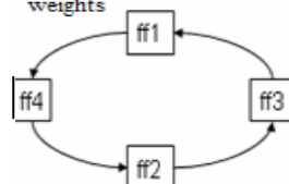
fig. 2b. final arrangement of the scan cells in the chain
