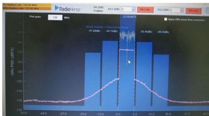
Figure 9: PAPR reduction using SDR
