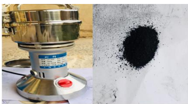
Figure 2: Grinding machine (to convert solid to powder)
