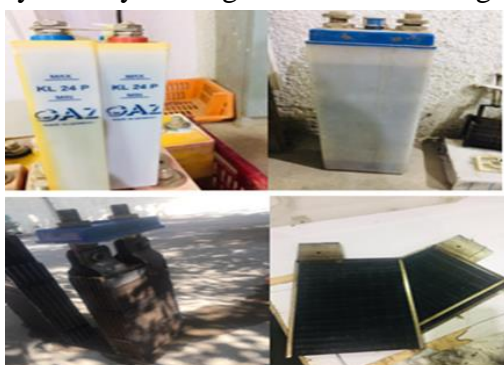
Figure 1: Disassemble the nickel-cadmium battery
