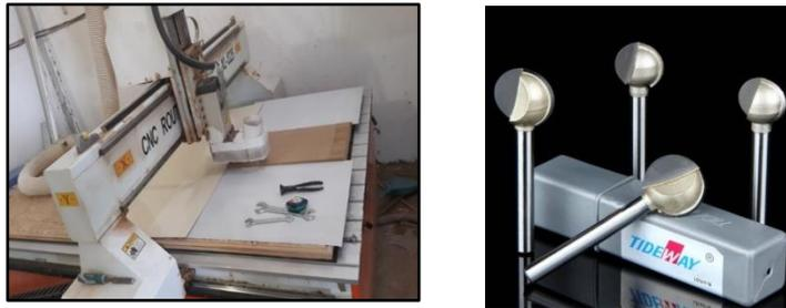
Figure (5): The CNC-Machine and sphere end screw
