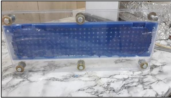
Figure (7): The mold for UPS casting
