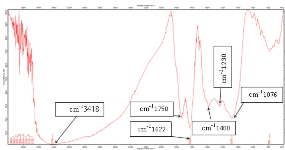
Figure 6. Transmission FTIR spectra of GO
