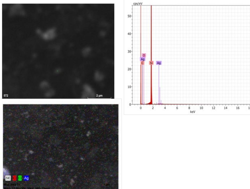
Figure 4. (A) EDX spectrum and (B) X-ray mapping images for the sample S5.
