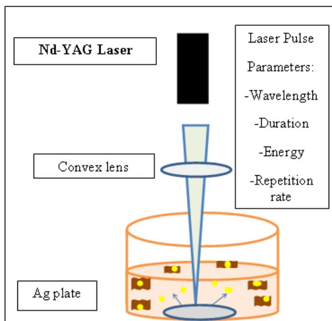
Figure 1. schematic illustrated that Ag NPs decorated on GO sheets at room temperature. The Ag NPs are tightly bonded to each GO sheet's surface, forming a hierarchical micro/nanostructure.
