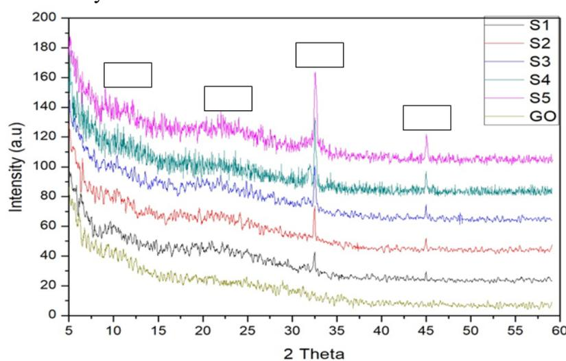
Figure 13. XRD pattern of GO and rGO-Ag NPs for five samples.
