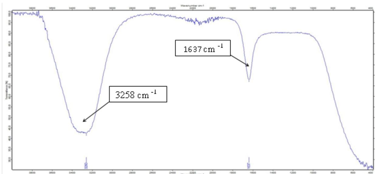
Figure 10. Transmission FTIR spectra of rGO-Ag S4
