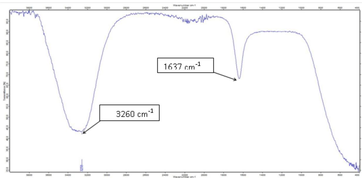
Figure 9. Transmission FTIR spectra of rGO-Ag S3
