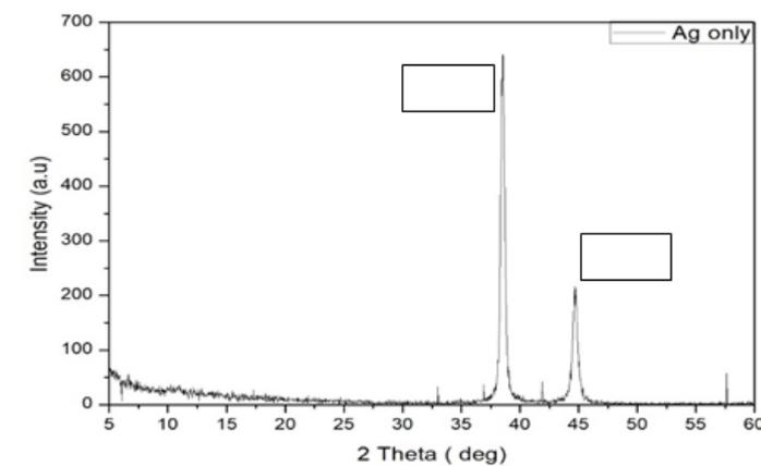
Figure 12. XRD pattern of Ag plate
