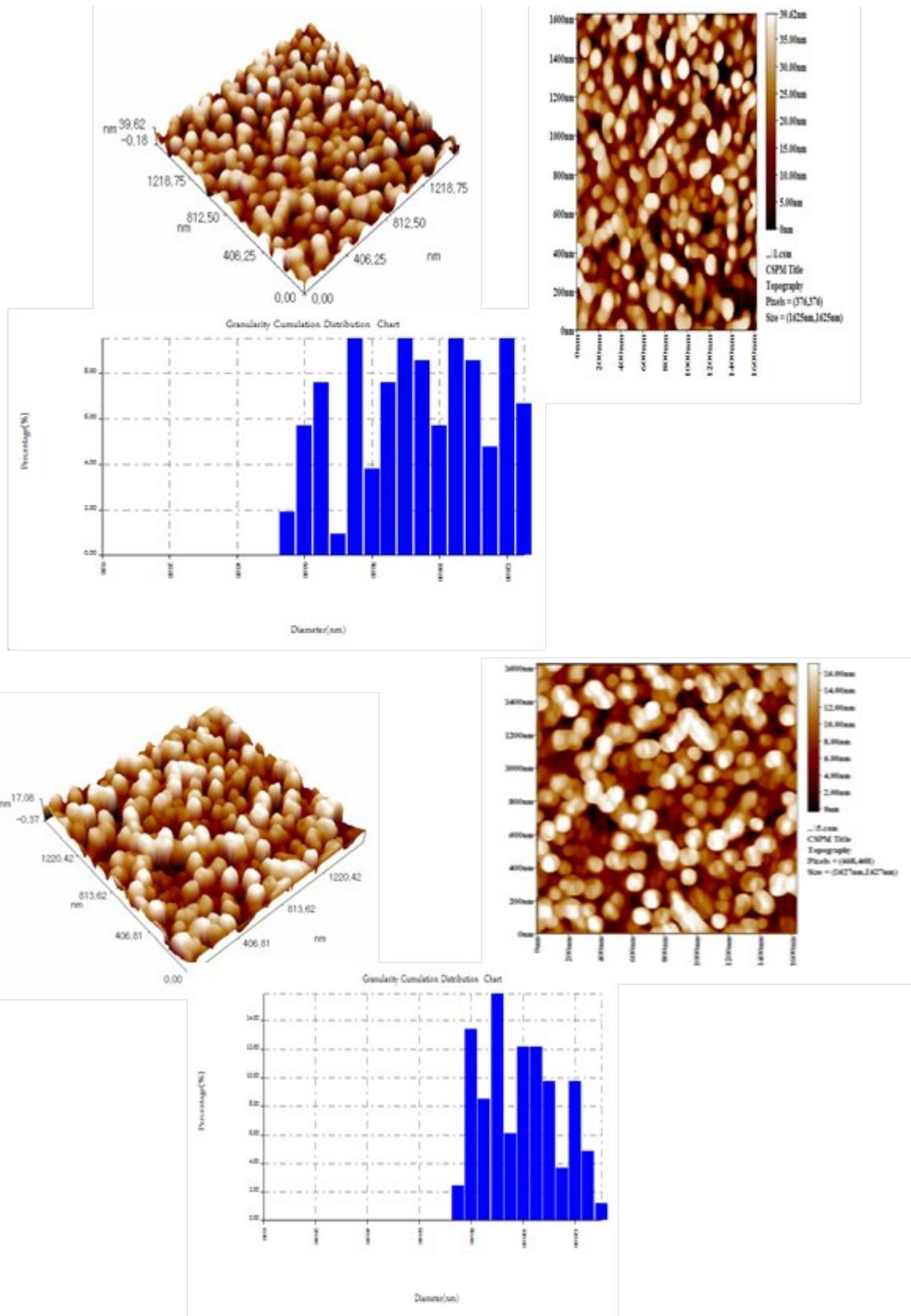
Figure 5. shows AFM images of the five samples structures in 1D, 2D and statistical distribution.
