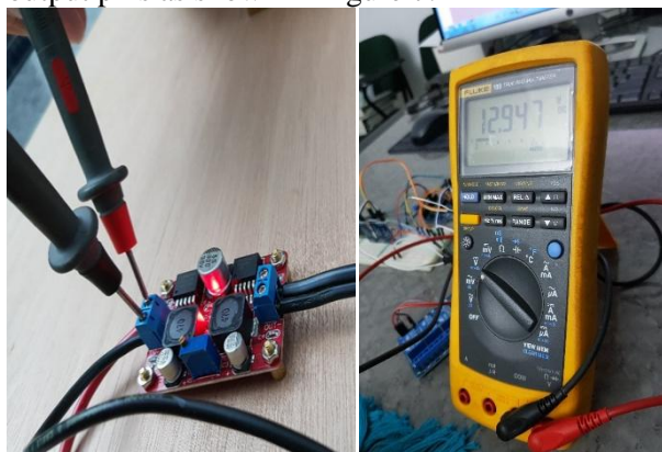
Figure 7. (a) the input pins of buck boost and input voltage result.
