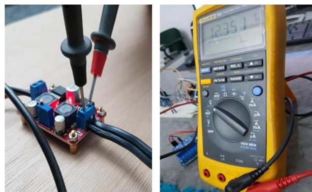
Figure 8. the output pins of buck boost and (b) output voltage result.
