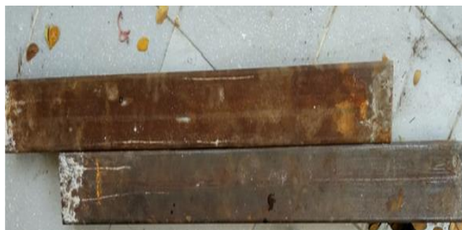
Fig.1 Rectangular Concrete Filled Steel tube beams
