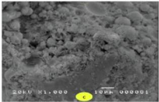
Microstructure of Geopolymer concrete
