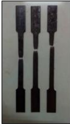
Figure 5: Based Specimen (Not Immersed in Salt Water) After Tensile Test
