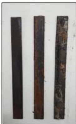
Figure 2: Formation of Corrosion After Period of Immersion (From Left: 20%, 40% & 60%)
