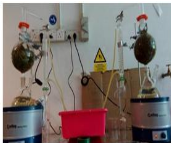
Figure 1: Extraction of essential oil through steam distillation
