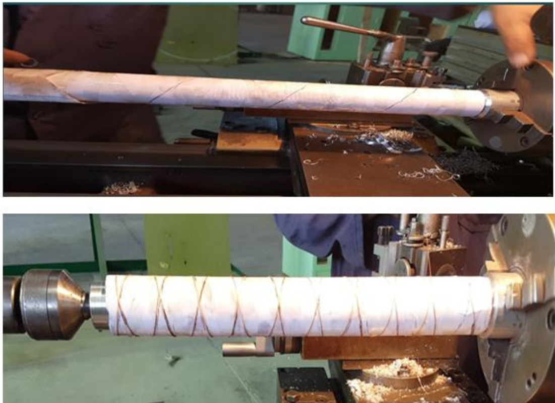
Figure (1.3): Delimit angle and winding fiber
