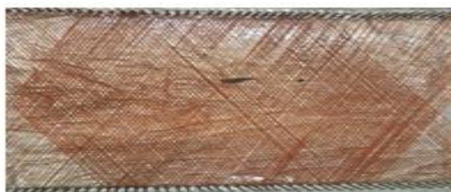
Figure (1.6): wax add on the wood mold
