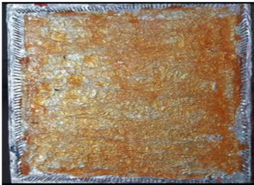
Figure (1.6): wax add on the wood mold
