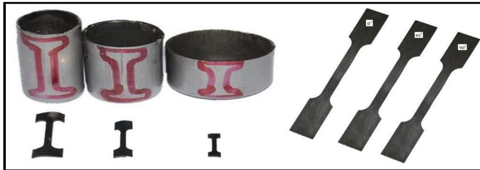
Figure:3 Shows the tensile samples were taken of the flat sheet and the cylindrical shape of the three stages
