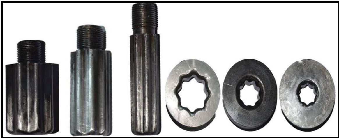
Figure: 5 The star punches and dies of the three stages drawing operation used.
