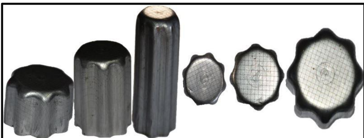
Figure: 7 The square grid at the wall and brace of the shape after the deep drawing of three stages.
