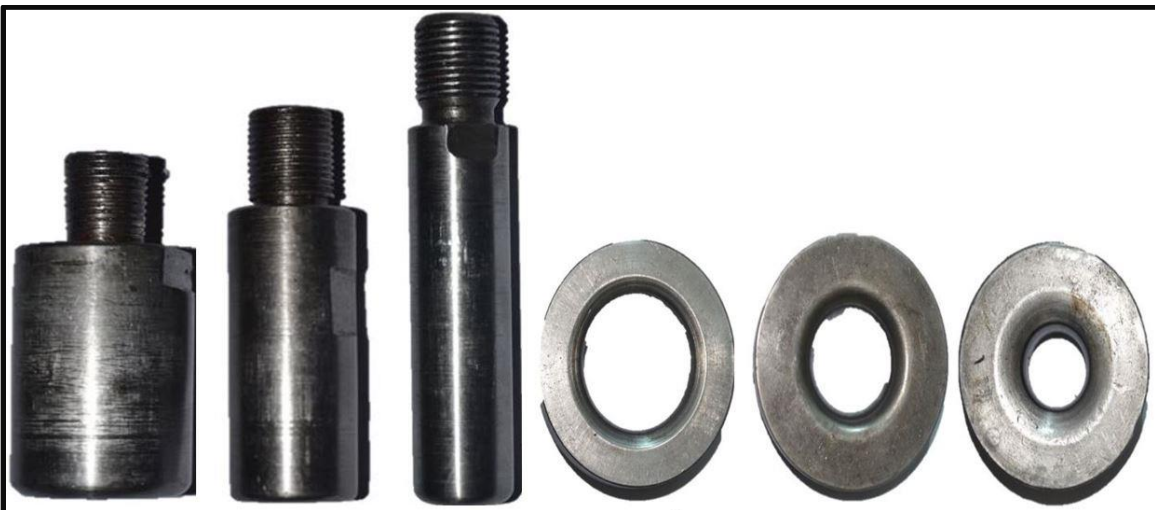
Figure: 6 The cylindrical punches and dies of the three stages drawing operation used.
