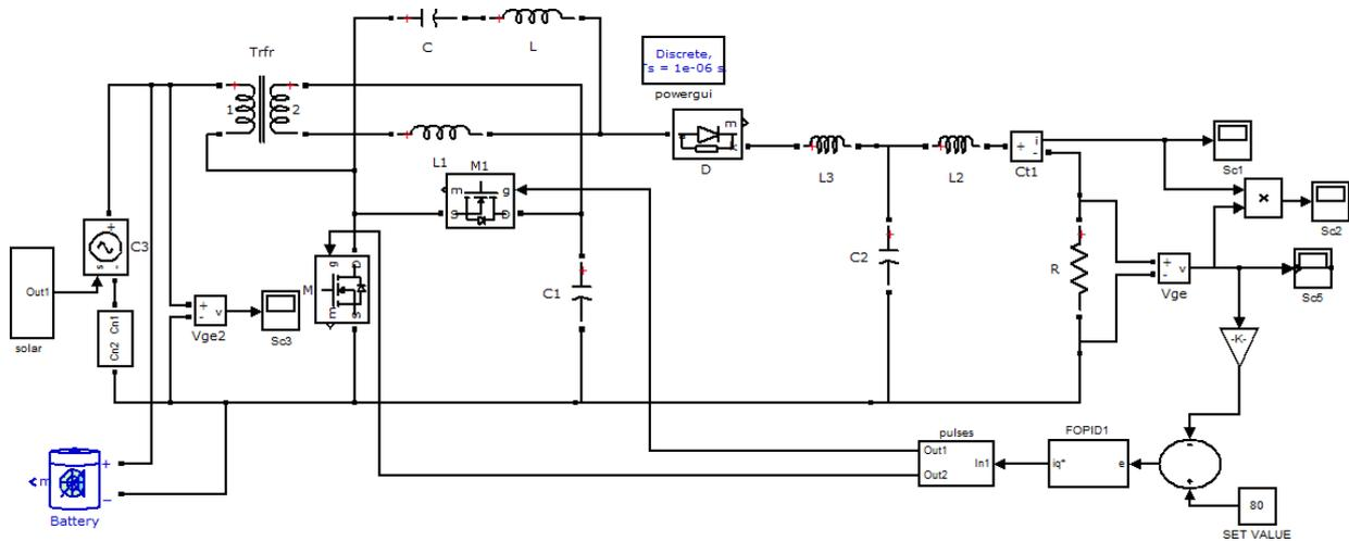
(a) Circuit diagram of PV and Battery based Modified SEPIC converter with closed loop FOPID controller
