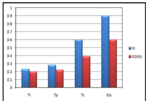
(g) Bar chart of PI and FOPID controlled system with Vref=80V
