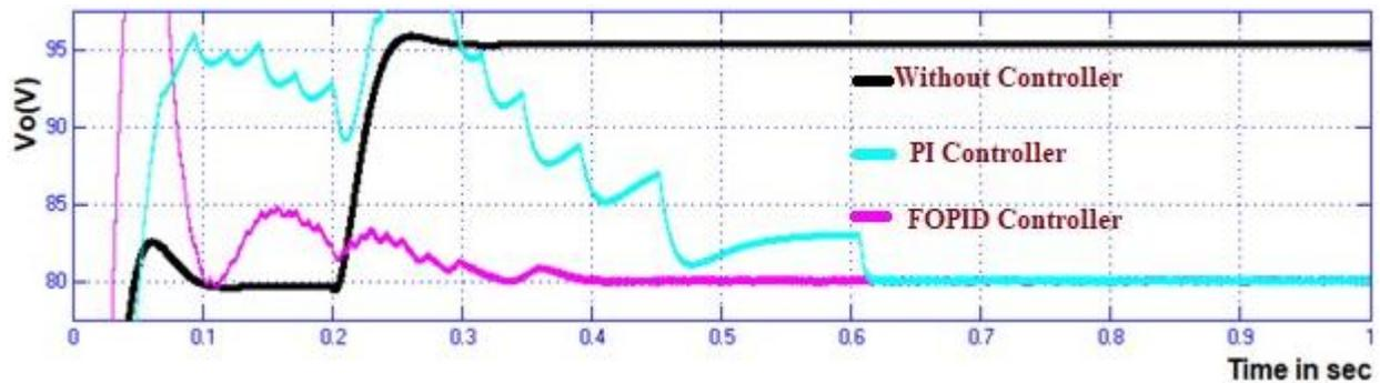
3.3 (f) comparison of output voltage regulation of without controller, with PI & FOPID controller
