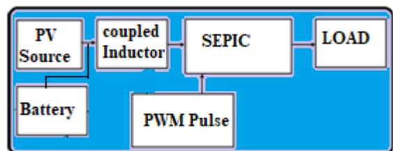
Fig. 1 (b) Coupled inductor based Modified SEPIC converter
