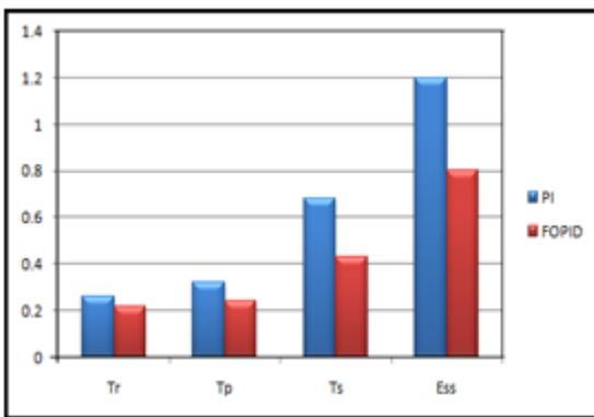
(h) Bar chart of PI and FOPID controlled system with Vref=85V
