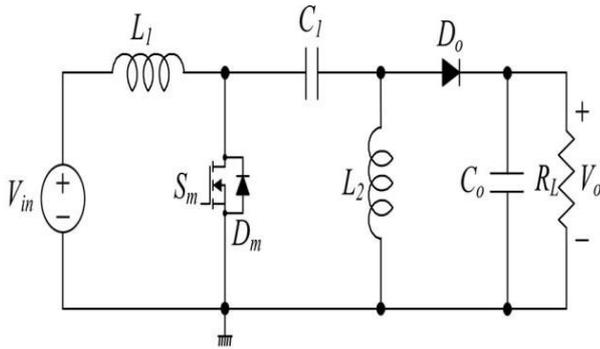
Fig. 1.1 Conventional modified coupled inductor based SEPIC converter
