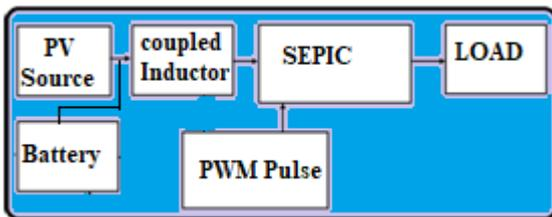
Fig. 1.2 Equivalent circuit of the modified coupled inductor based SEPIC converter
