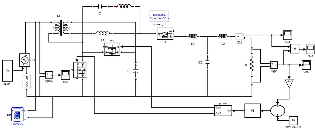
3.2 (a) Circuit diagram of PV and Battery based Modified SEPIC converter with closed loop PI controller
