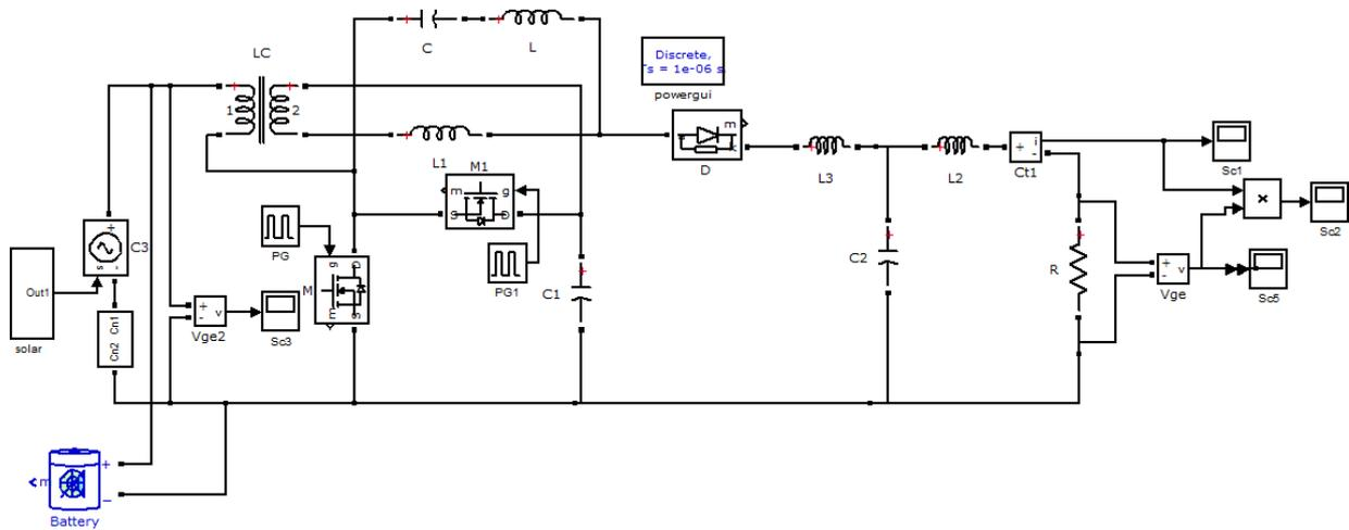
Fig. 3.1 (a) Circuit diagram of PV and Battery based Modified SEPIC converter with Open loop source disturbance
