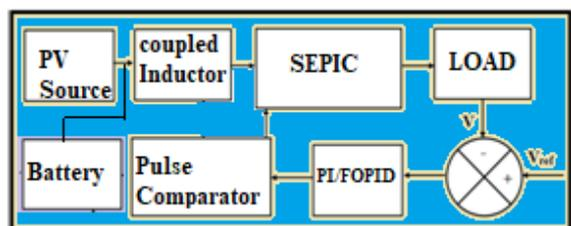
Fig. 1 (c) Closed loop controlled coupled inductor based SEPIC with renewable system
