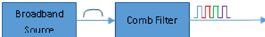
Fig. 3 General overview of comb filter based multi-wavelength laser
