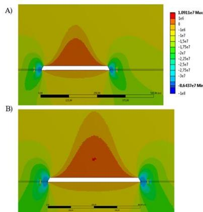
Fig 2 The impact of panel width on the tensile zone in the rocks above the mine void: A)  $l = 300$  m; B)  $l = 400$  m
