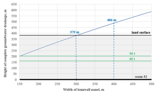
Fig 1 The impact of panel width on the height of complete groundwater drainage
