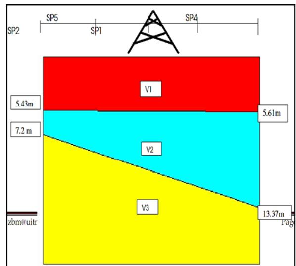
**Fig 3. Soil profile at line D-D'**
