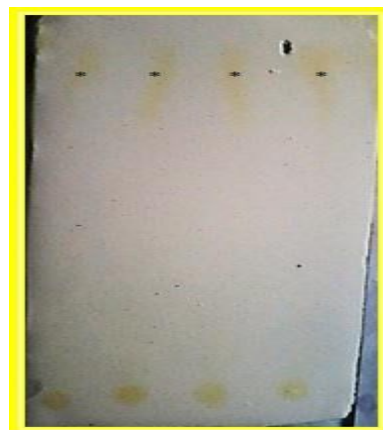
Fig 6: Thin Layer Chromatogram Of EPS Isolated From The Bacterial Strain (The Separated Spot Has Been Marked With An *)
