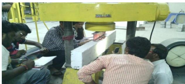
**Figure 2.2 Calculation of strain at compression and tension face using damec gauges.**
