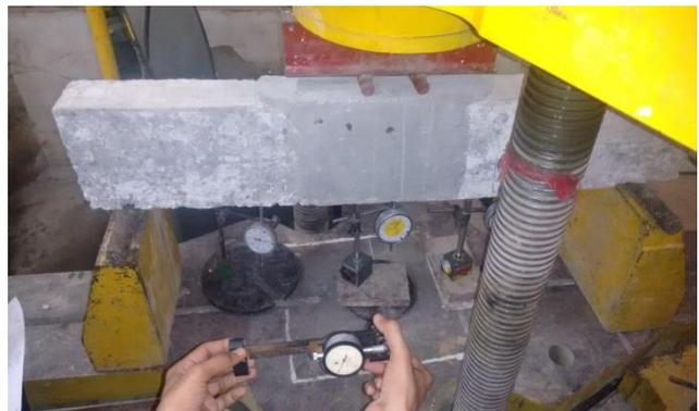
**Figure 2.6 Failure of retrofitted beam after testing**
