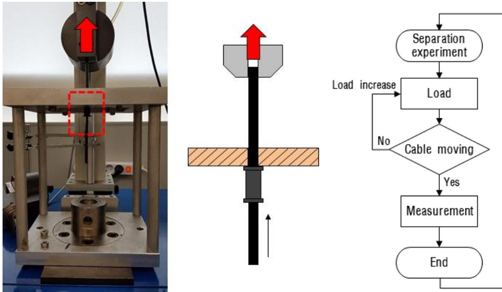
(a) Schematic diagram of separation force experiment (b) Flowchart of separation force experiment
