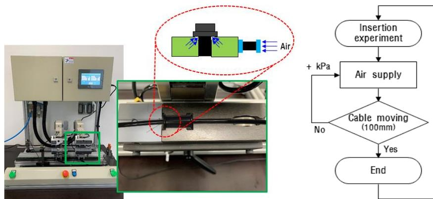
(a) Airjet insertion process equipment and schematic diagram for air supply (b) Insertion force experiment flowchart
