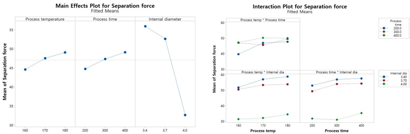
(a) Main effects plot for separation force (b) Interaction plot for separation force
