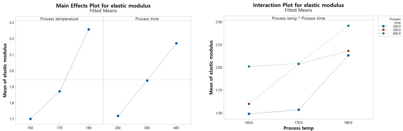
(a) Main effects plot for elastic modulus (b) Interaction plot for elastic modulus
