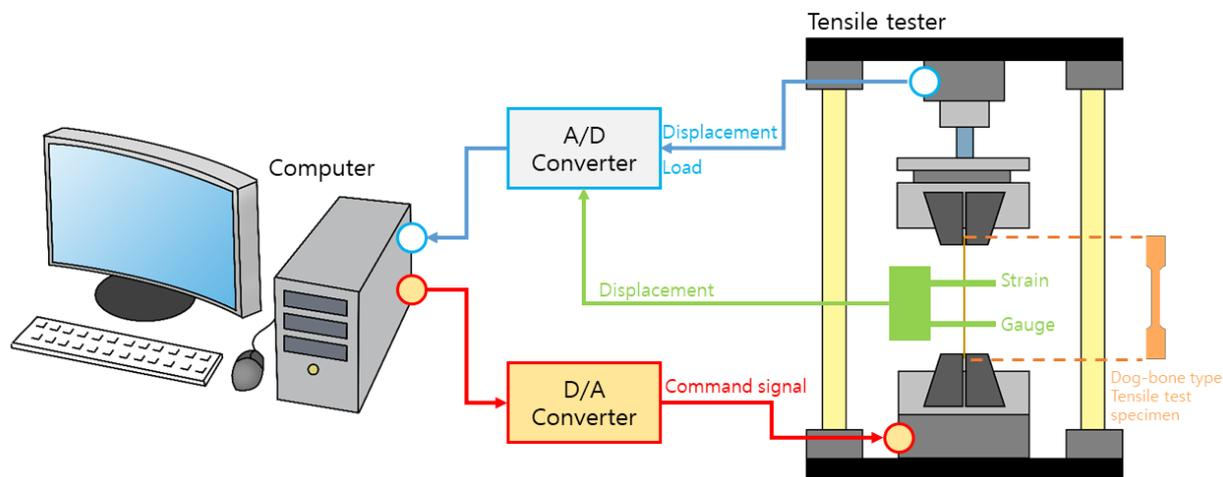
Figure 2. Schematic diagram for rubber tensile strength test.
