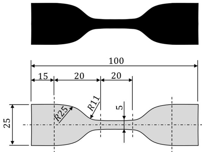
Figure 1. Specimen specification for rubber tensile strength test.
