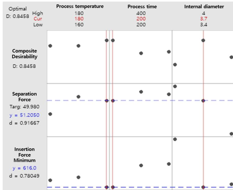
Figure 9. Parameter optimization results using response optimizers.
