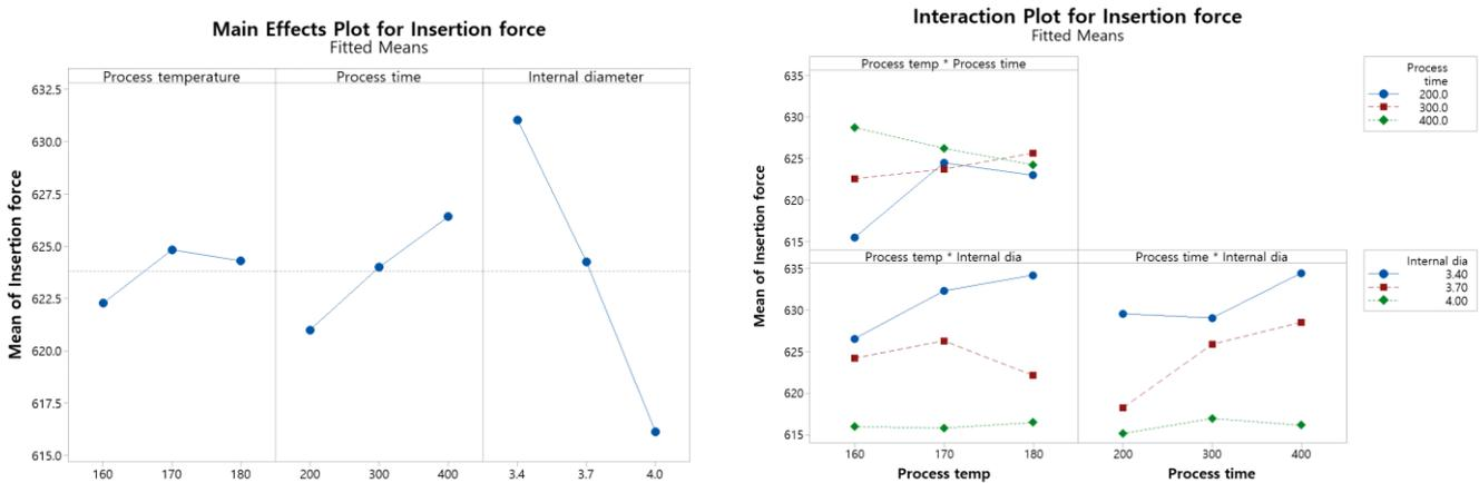
(a) Main effects plot for insertion force (b) Interaction plot for insertion force
