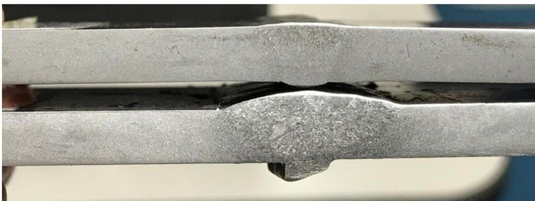
**Figure 13. Sectional appearance of the etched specimens by GTAW and FCAW process.**
