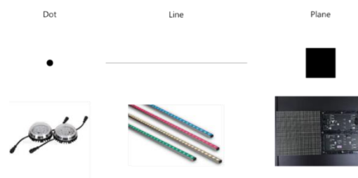
Figure 1. Classification by type of general LED module
