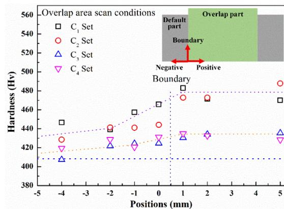
**Figure 2. Variation of Vickers hardness with positions**
