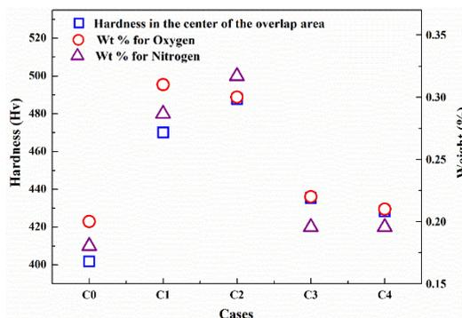
**Figure 4. Comparison between hardness in the center of the overlap area and the amount of oxygen/nitrogen with the energy density of the overlap laser scanning**
