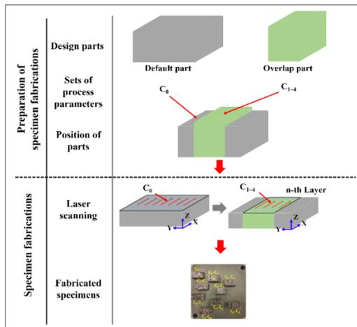
**Figure1. Schematic diagram for specimen fabrication in the proposed method**
