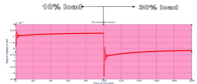
Figure 2.12(b) Frequency variation in area1 with PI Controller at 10% and 30% load
