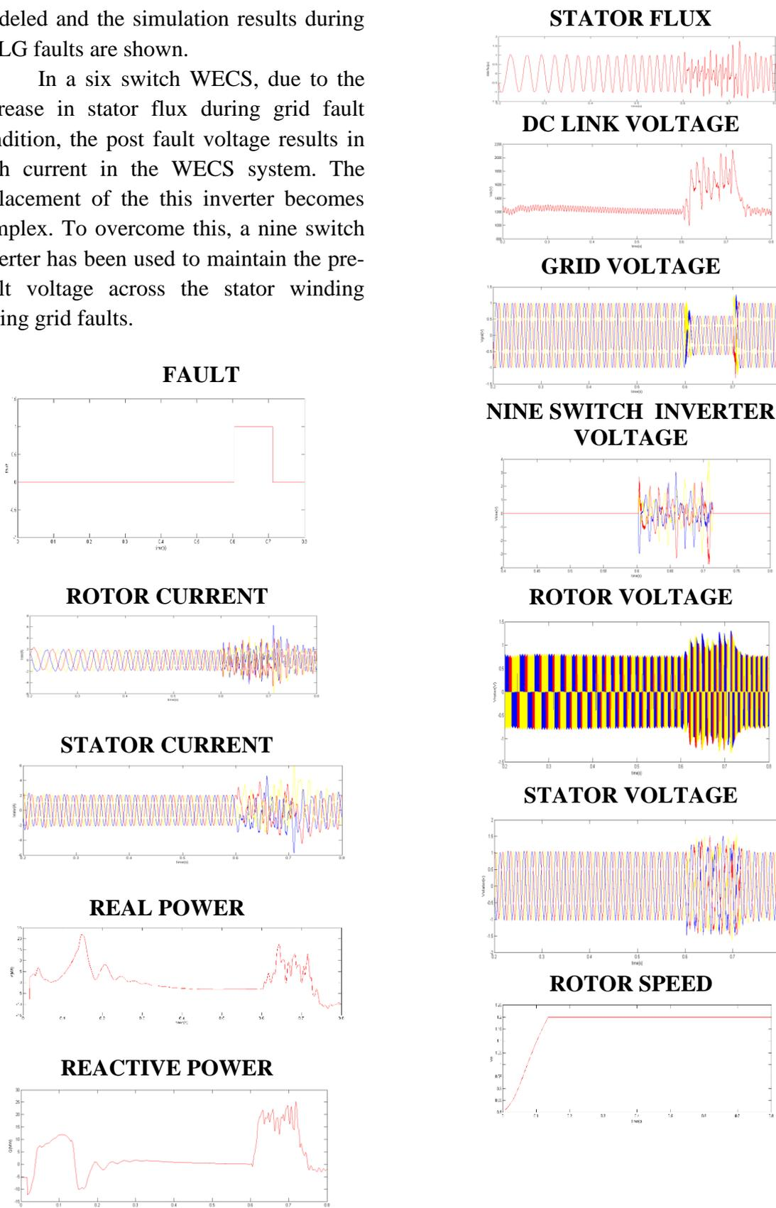
**Fig 6 Simulation result of NSI fed DFIG based WECS with PI Controller during LLLG fault**
