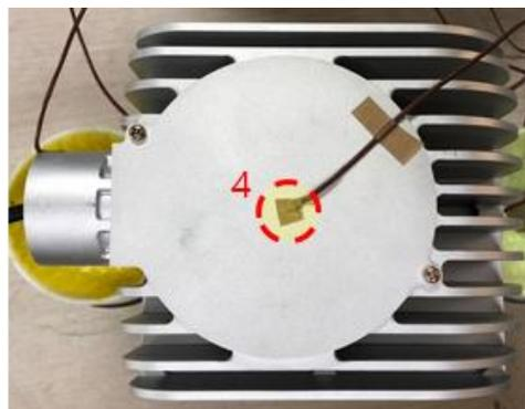
[The point of measurement of heat sink (Back)]
